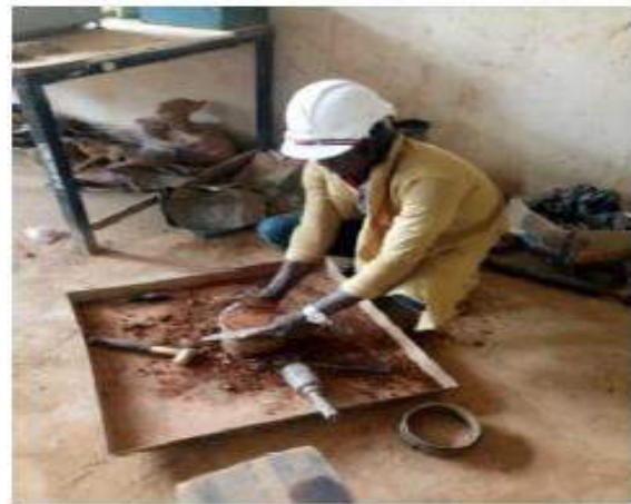
Figure 3: Compaction test on the clay soil
