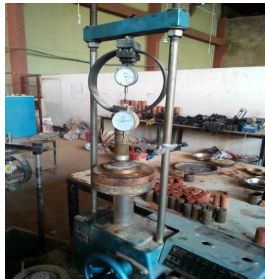
Figure 2 Unconfined compressive strength test
