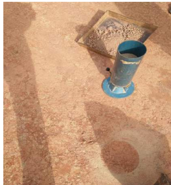
Figure 3: In-situ density test
