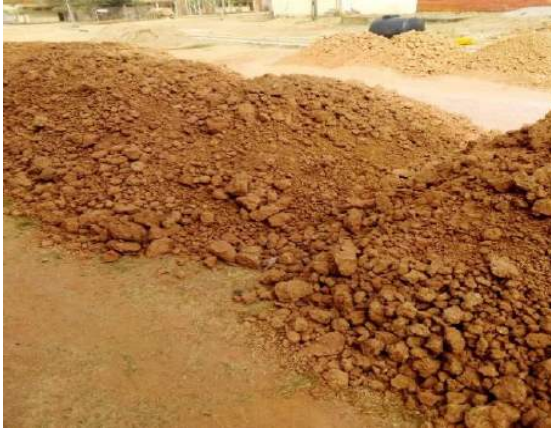
Figure 1: Pile of laterite Soil
