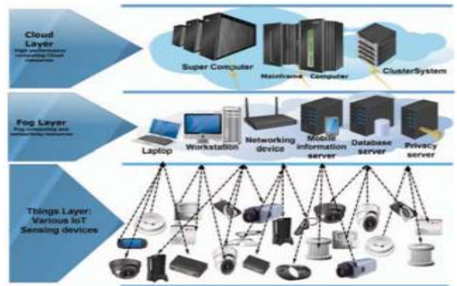
Figure 3. IoT-Fog Cloud use case for 5G Architecture
