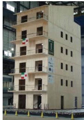
Fig. 1: Seven-story CLT house tested at E-Defense Laboratory in Miki (Source; Mohammad et al. , 2015)
