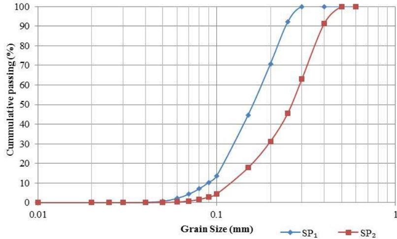
**Figure 6: PSD analysis of SP<sub>1</sub> and SP<sub>2</sub> by CT-scanning (Olawuyi, 2015)**
