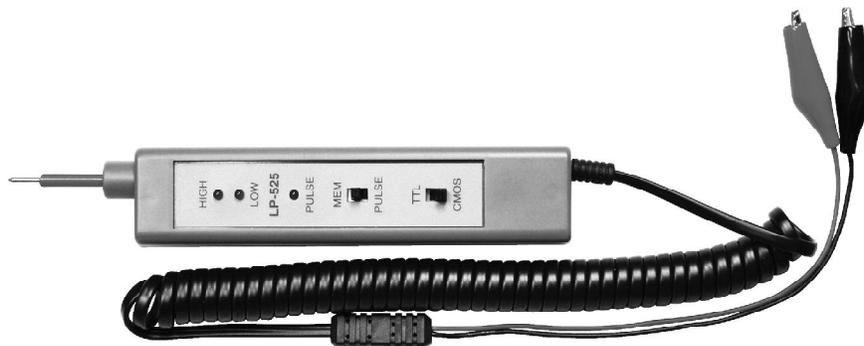
**Figure 2.19: Model Logic Probe**
