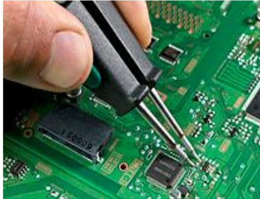
**Figure 2.38: Soldering Tweezers**
