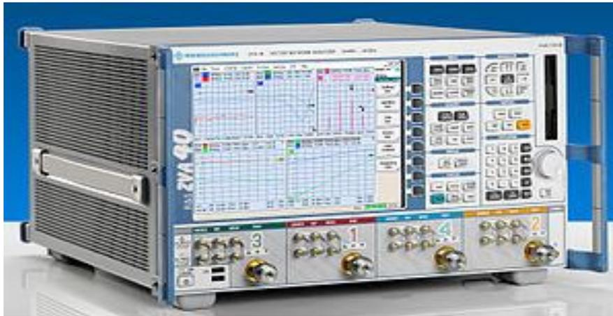
**Figure 2.22: A Typical Network Analyser**
