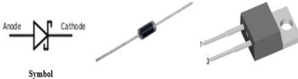
**Figure 1.13: Circuit Symbol and Packaged Schottky Diodes**
