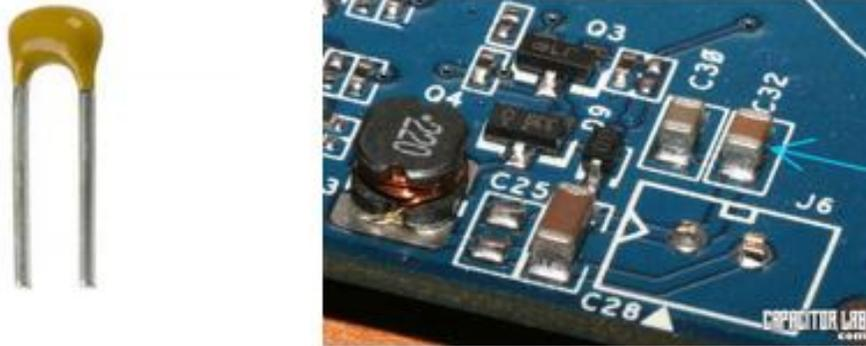
**Figure 1.6: Through-Hole and Surface-Mounted Ceramic Capacitors**
