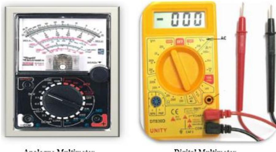
**Figure 2.1: Analogue and Digital Multimeters**
