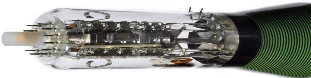
Figure 4.5: Photograph of a Typical Cathode Ray Oscilloscope Tube Source: Carl (2010)
