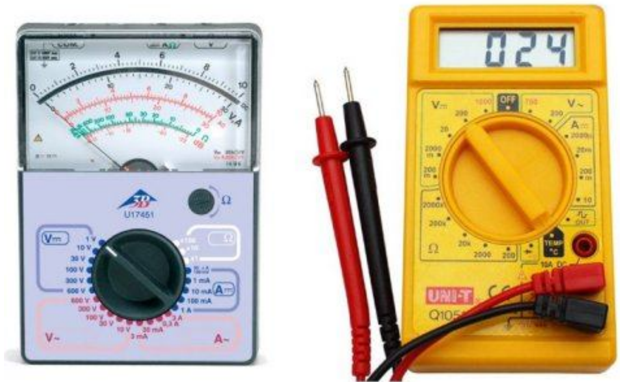
Figure 2.1: Features of Analogue and Digital Multimeters Source: www.technologyuk.net
