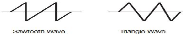
Figure 4.13: Saw-tooth and Triangular Waves
