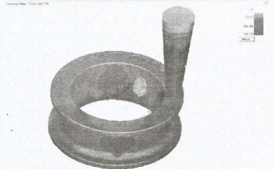
Figure 11: 3D plot of the cooling rate for the final simulation
