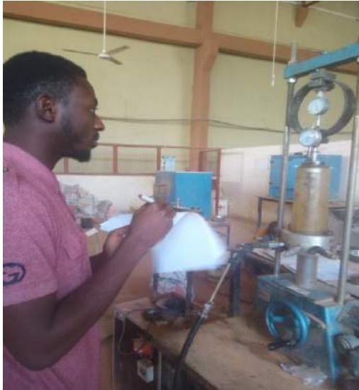
Plate 1: Consolidated undrained test on samples
