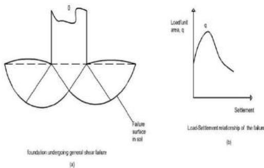
Figure 1: General shear failure (Das, 2007)
