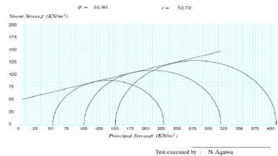
Figure 5: Mohr circle diagram for LGB samples
