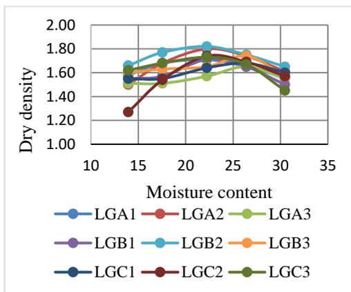
Figure 3: Sample compaction curve
