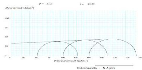
Figure 6: Mohr circle diagram for LGC samples
