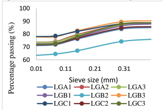
Figure 2: Grading curve of samples
