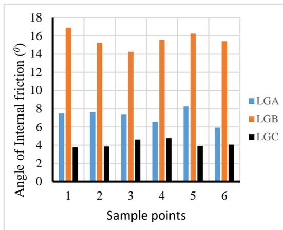
Figure 6: Ang. of Inter. friction of samples from clusters A, B and C
