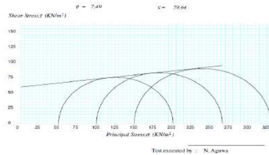
Figure 4: Mohr circle diagram for LGA samples
