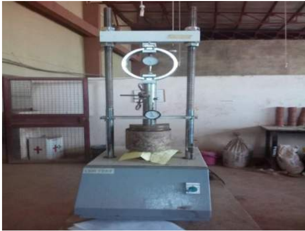
Plate II: California Bearing Ratio test of samples
