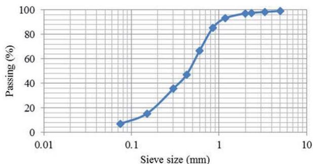
Fig. 3. Particle size distribution curve for RHA
