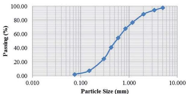
Fig. 1. Particle size distribution curve for fine aggregates
