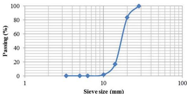
Fig. 2. Particle size distribution curve for coarse aggregates
