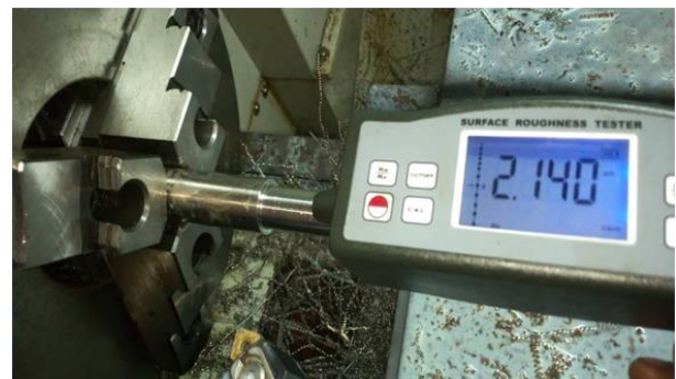
Plate III: Set up for measurement of surface roughness of turned surface.
