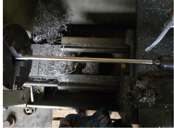
Plate I: Experimental set up for orthogonal turning process showing all components
