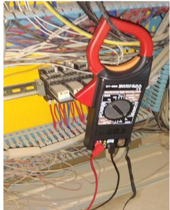
Plate II: Experimental set up for measurement of current and voltage using clamp meter
