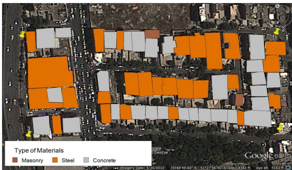
Fig 9. Digitized photo of building targets by MapInfo based on material of construction
