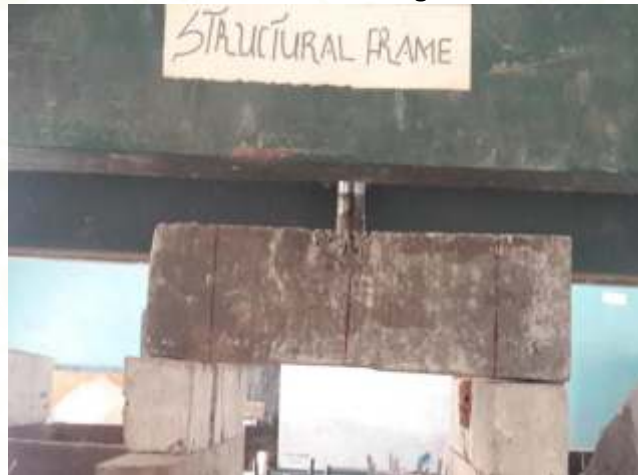
Figure 4a. Beam under three point load
