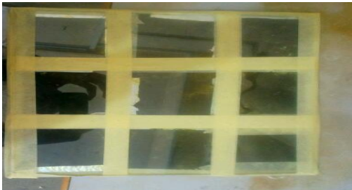
Plate; IV Solar photovoltaic module consisting of nine series connected solar cells
