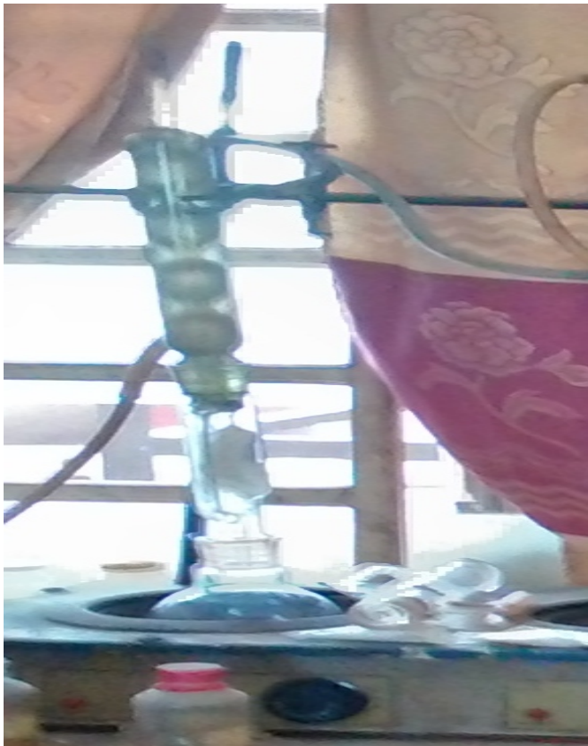
Plate 1: Electromantle ME Soxhlet extractor in WAFT Department Federal University of Technology Minna.
