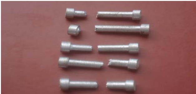
Plate I: Aluminium Cast Samples after Tensile Tests
