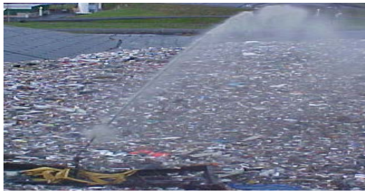
Fig. 15: Innovative bioreactor liquid sprayed on waste
