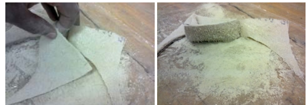
Fig. 7: GCL sliced open to remove bentonite material
