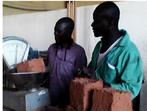
Plate II: Weighing of Coir-Laterite blocks
