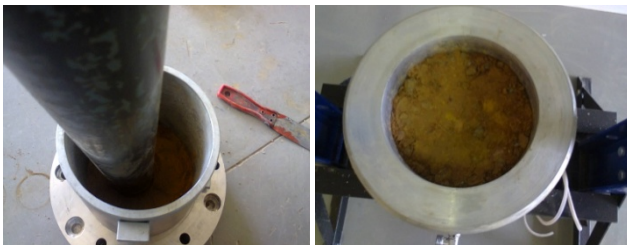
Fig. 5: (a) Standard proctor compaction of soil (as subsoil) (b) Lightly compacted subsoil in bucket section
