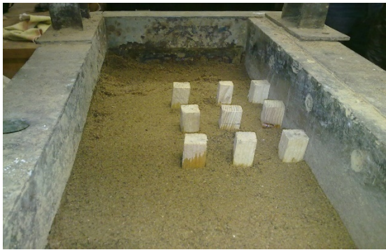
Fig. 3: Modelled Test Piles Bored into the Soil
