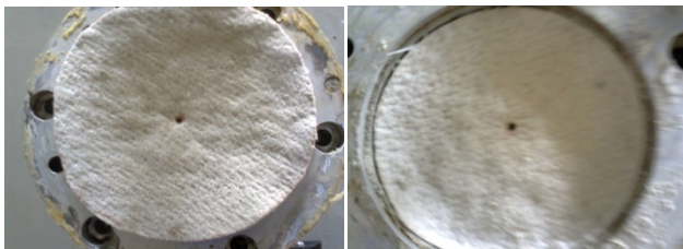
Fig. 9: (a) 24mm thick GCL placed over 160 mm diameter subgrade with headspace to accommodate swelling
