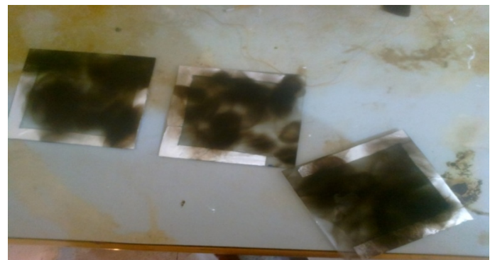
Plate III: Cathodes formed by burning the aluminium foil coated transparent glasses on a candle flame.
