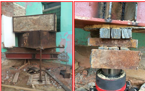
Fig. 6: Load Test Modelled Test Piles
