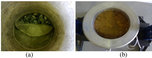
Fig. 7: (a) Hydrated geotextile on porous stone to prevent outlet clogging (b) Lightly rammed BS to simulate loosed subsoil
