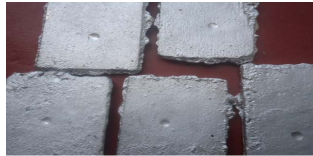
Plate II: Aluminium Cast Samples showing Indentation of Hardness Tests
