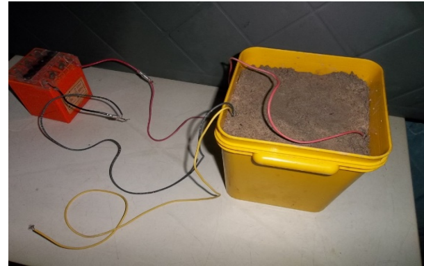
Fig.1: Impressed current cathodic protection setup.
