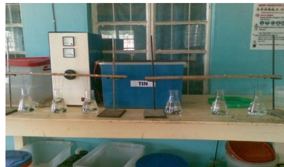
Plate 2: Corrosion test set-up
