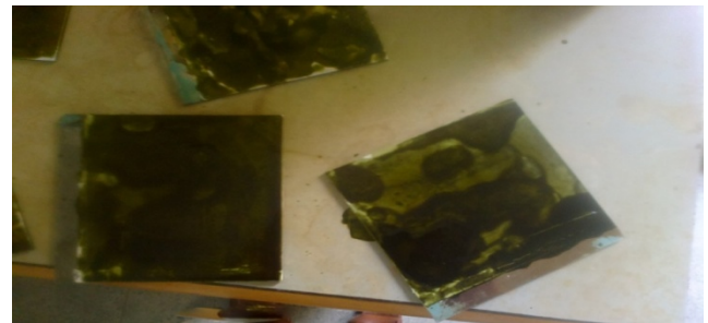
Plate II: The anodes formed by staining the \text{TiO}_2 coated glasses with natural dye
