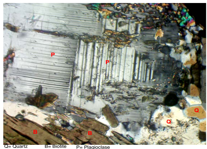
Q= Quartz B= Biotite P= Plagioclase Plate 1b: Under cross polarize light (Magnification X40)
