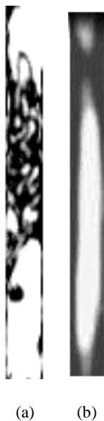
Figure 6: comparison of contours of phase distribution, same inlet velocity condition for (a) CFD (b) ECT. The liquid and gas phases are represented by dark and light colours, respectively
