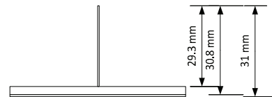
Fig.2. Side view of the monopole antenna
