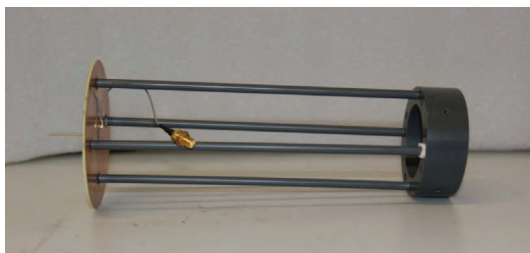
Fig.5. Monopole antenna mounted on the support pole.
