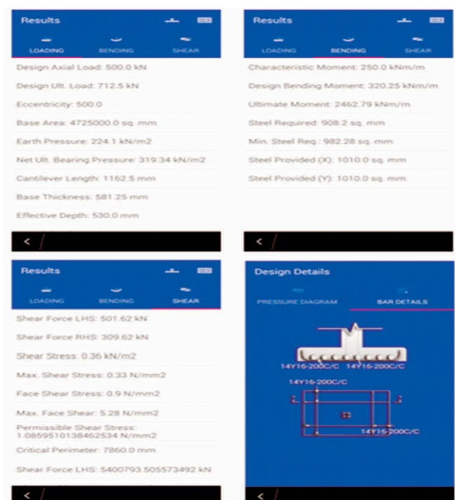
Plate 2. Result for Axially Loaded Pad Foundation Subjected to Moment using the Android Mobile Application
