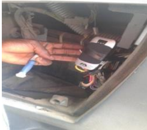
Figure 3: Installation of the AVLE in the bus
