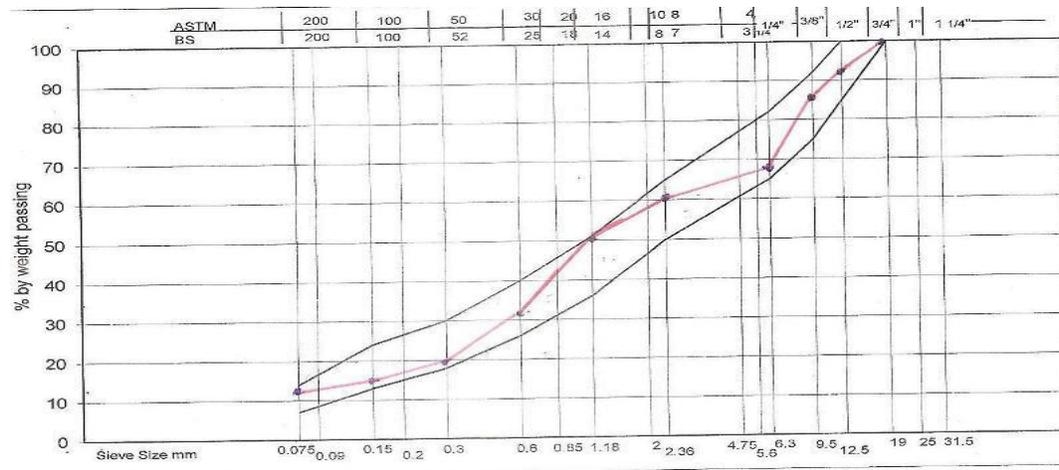
Figure 1a: Obtained from the Combined Gradation of Natural Aggregate.
