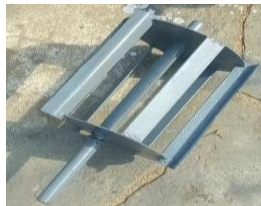
Plate2. The horizontal type weeding blade
