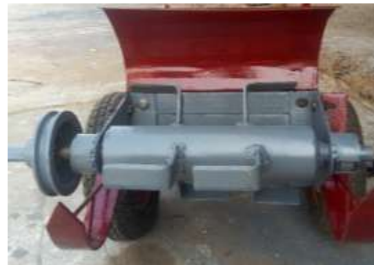
Plate1. The finger type of weeding blade
