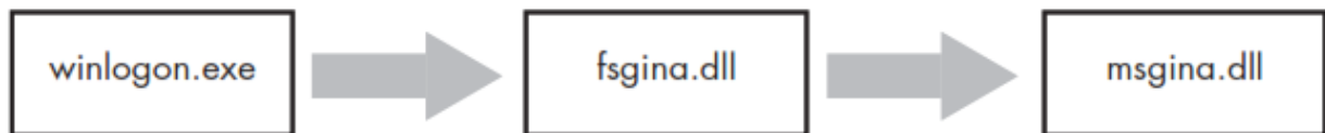
Fig. 5.6: Malicious fsgina.dll sits in between the Windows system files to capture data
