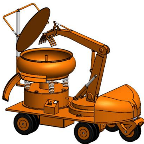
Figure 11: The electro-mechanical system model for the intelligent mobile metal scrap separating and cleaning system
