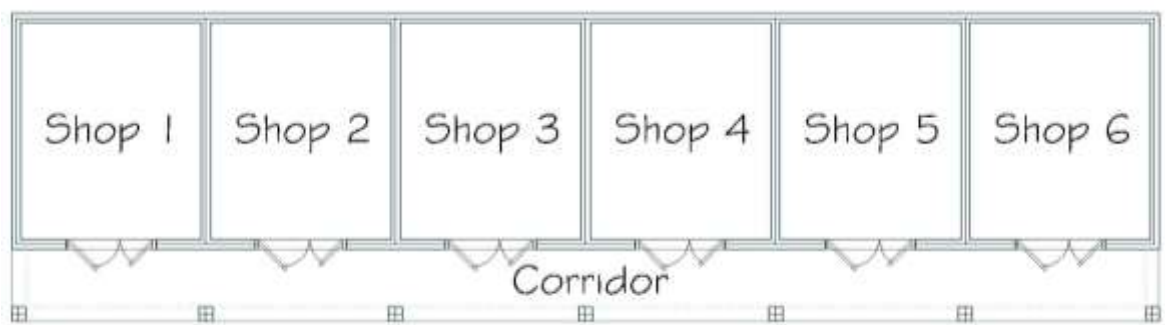
Figure 3.4: Typical ground floor plan of the lock-up shops in Wuse market. Source: Field work (2017).
