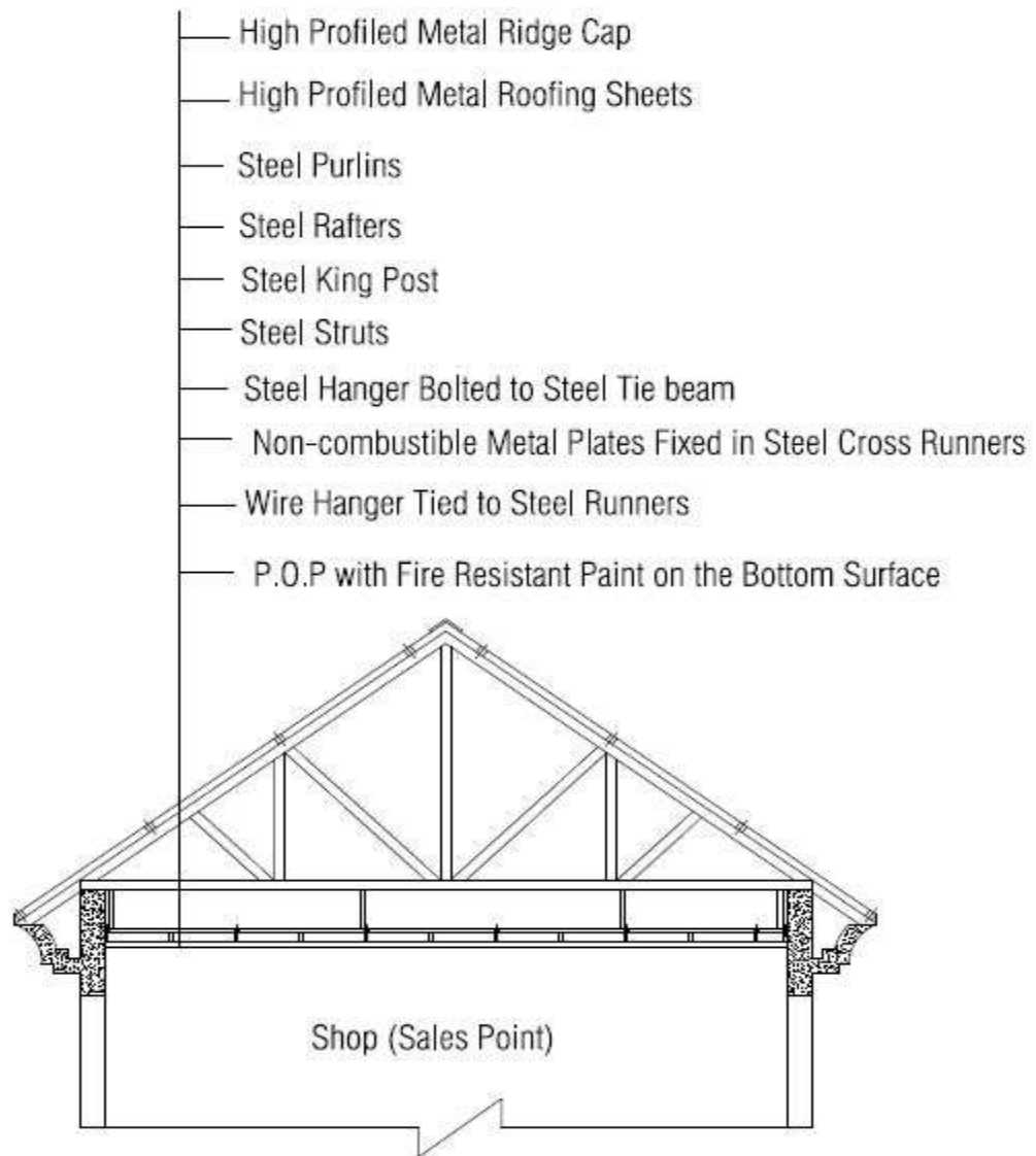
Figure 5.7: Section of a proposed shop building revealing composite ceiling arrangement connected to the roof structural members.
