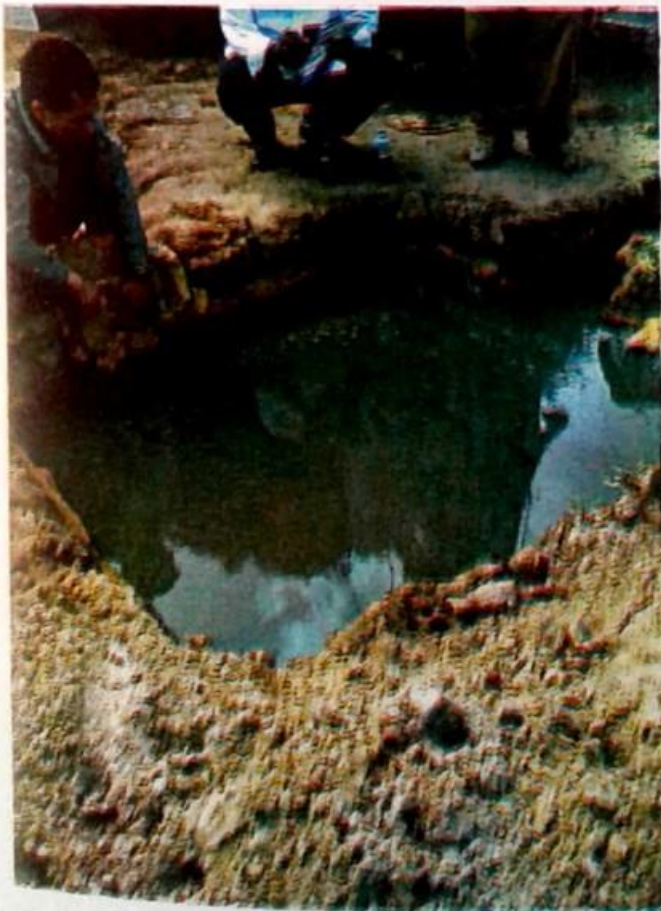
Head of Geological Operation of the Shekang Group of China observes oil slicks on water during a second drilling of shallow well at Kudu in June 2014. Drilling was entirely water-based. No diesel nor any chemical used.
