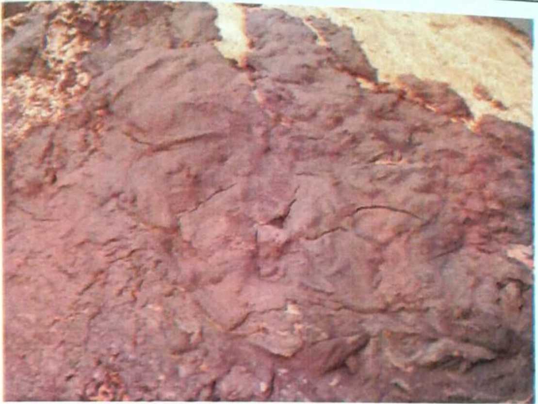
Dark~coloured muds / shales (potential petroleum source rocks) recovered at shallow depths in the Kudu-1 well
