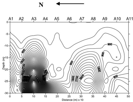
Fig.4: Geoelectric Vertical section along Profile A along Profile B
