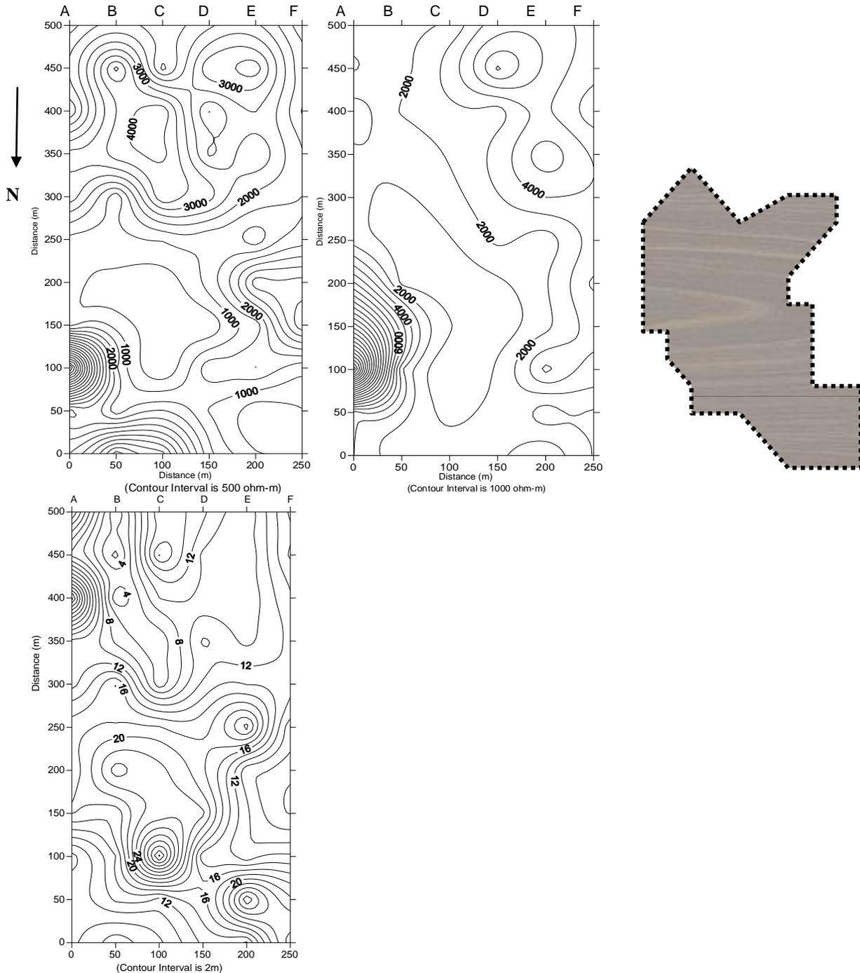
Fig. 13, 14 and 15: Iso-resistivity contour Map at 20m Depth, 30m Depth and Depth to Basement contour Map Respectively
