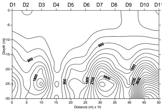
Figure7: Goelectric Vertical section along Profile D (Contour Interval is 300Ωm)
