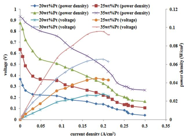
**Fig. 13** Polarization curve of a single cell operated at 25 °C with H<sub>2</sub>/O<sub>2</sub> ratio of 1:2
