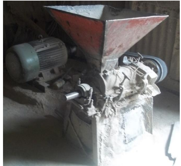
Fig. 2 Local steel friction mill without Aspiration Unit
