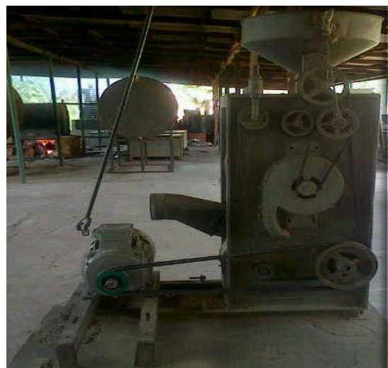
Fig. 3 Rubber Rolls Huller with Aspirator Unit
