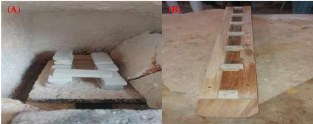
**Plate III: (A) Trial bars from beneficiated kaolin and (B) Mould**
