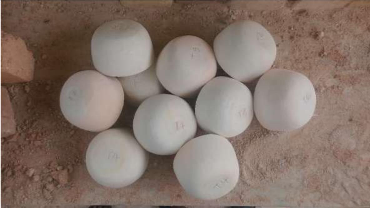
**Plate XIV: Fabricated Kaolin Filter Pots at different Proportions of Sawdust and Kaolin**
