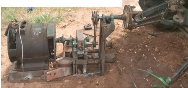
Fig. 2: Completed PTO Actuated electricity generation system connected to the tractor
