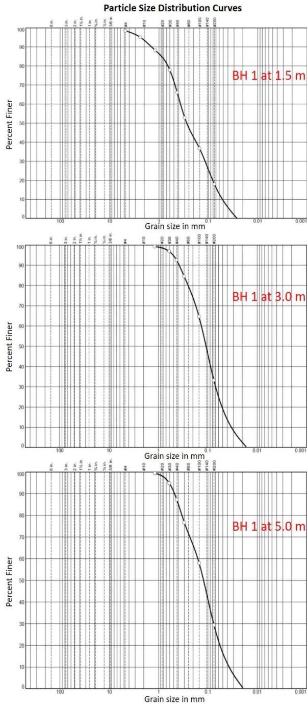
Figure 4: Results of Particle Size Analysis in Soil Samples Taken from BH 1.
