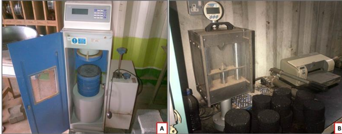
Figure 2: A. The UCS, and B. Point Load Test (Diametrical Test) Machines at the Setraco Construction Company Laboratory in Abuja, Nigeria (with the permission of the Company).
