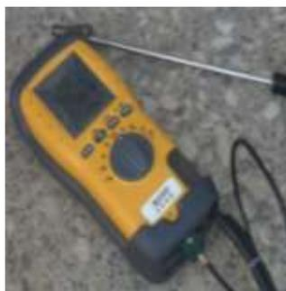
Fig.1. IMR1000-3/4 Combustion Gas Analyzer
