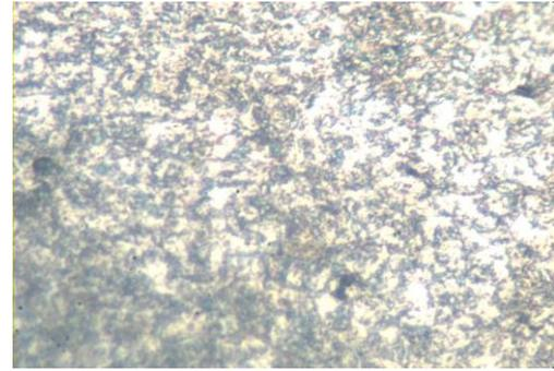
**Plate 7:** Micro graphs after case hardening with the mixture of charcoal and sea shells at 950 °C at magnifications of 600, and two hours soaking time. Ferrite transformation also favoured with finer grains.
