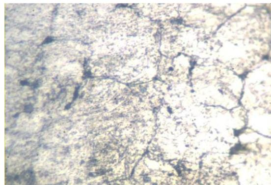
**Plate 3:** Micro graph after case hardening with charcoal at 900 °C at magnification of 600, and three hours soaking time. Transformation of Ferrite to iron carbide was favoured by significant uptake of more carbon from the charcoal.
