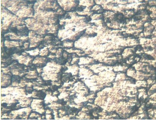
**Plate 4:** Micro graphs after case hardening with sea shells at 900 °C ×600, and holding time of three hours. Coarser grains of Ferrite with interstitial iron carbide.
