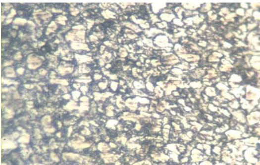
**Plate 6:** Micrographs after case hardening with the mixture of animal bone, charcoal and sea Shells at 950 °C at magnification of 600, and two hours soaking time. Finer grains with few transformation from ferrite to iron carbide favoured by carbon uptake.
