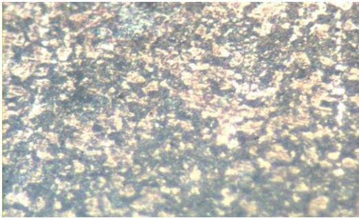
**Plate 5:** Micro graphs after case hardening with sea shells at 950 °C at magnification of 600, and holding time of two hours. Ferrite grains with interstitial carbide.
