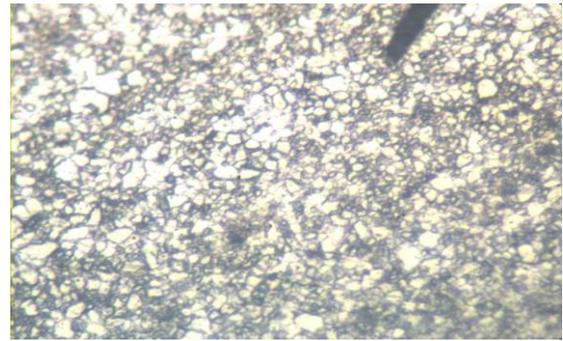
**Plate 1:** Microstructure of the mild steel before heat treatment × 400; Ferrite (Whitish) and iron carbide (Fe<sub>3</sub>C) phases clearly shown in an intermixed assemblage.
