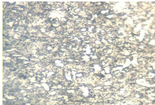
**Plate 2:** Micro graph after case hardening with animal bone at 950 °C at magnification of 600, and two hours soaking time. Ferrite is still distinctly seen untransformed.
