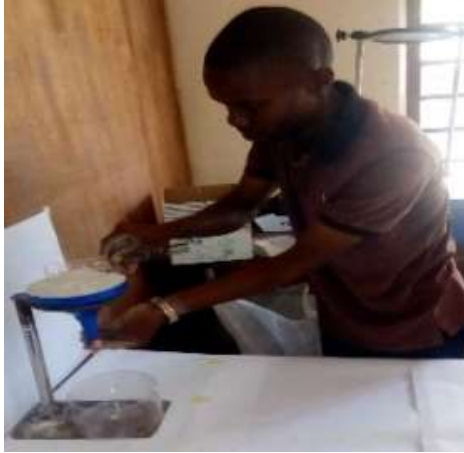
Plate VI: Test procedure for density test of powder materials (filler).
