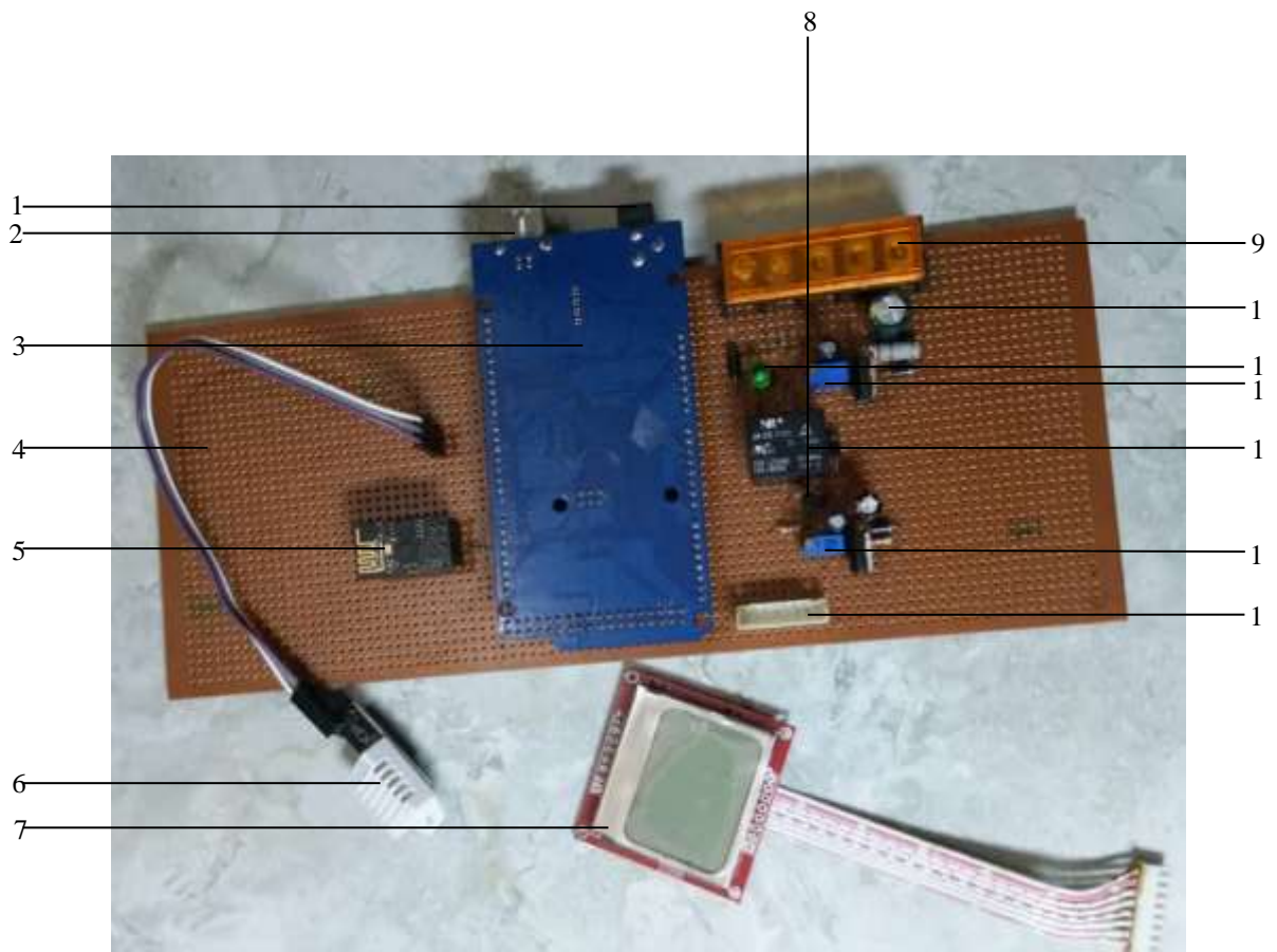
Plate I: Components mounted on vero board
