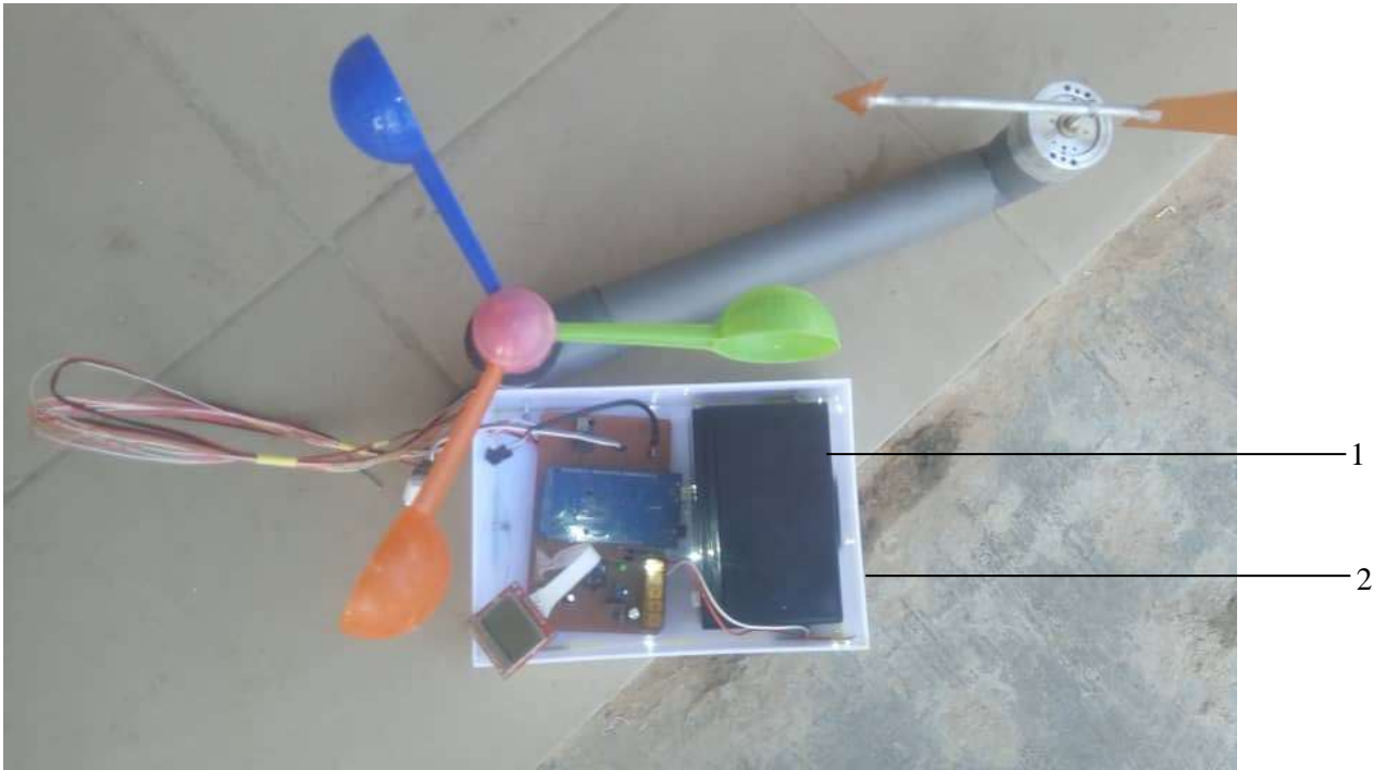
Plate III: Casing interior of the designed and constructed microcontroller-based weather station
