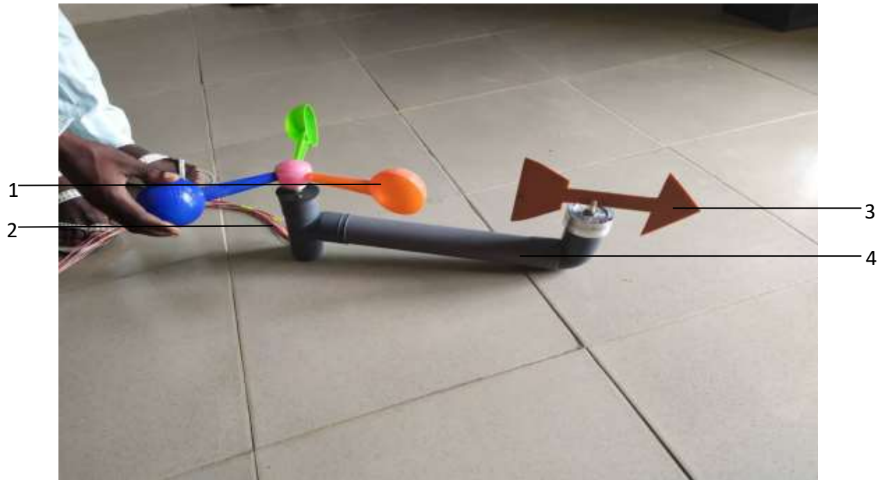
Plate II: Locally constructed anemometer and wind vane
