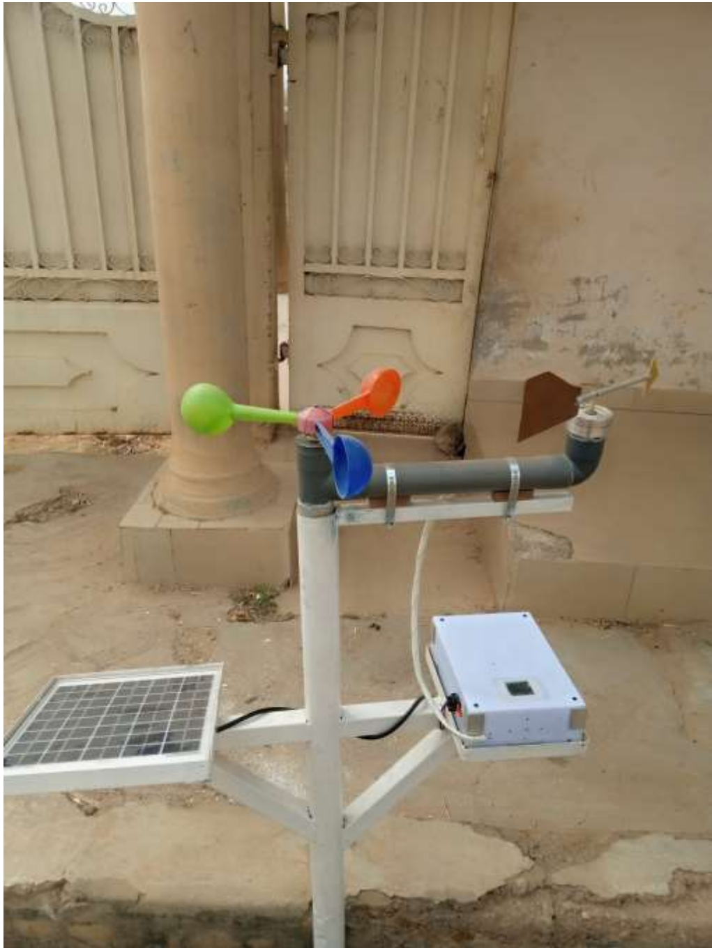
Plate V: The Set-Up of the Real-Time, Solar-Powered Microcontroller-Based Weather Station.
