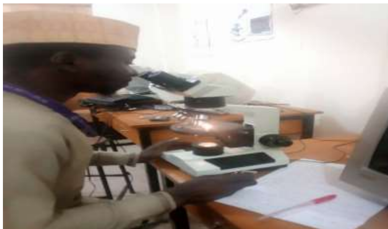
Plate II: Photograph of a petrological microscope used for thin-section studies
