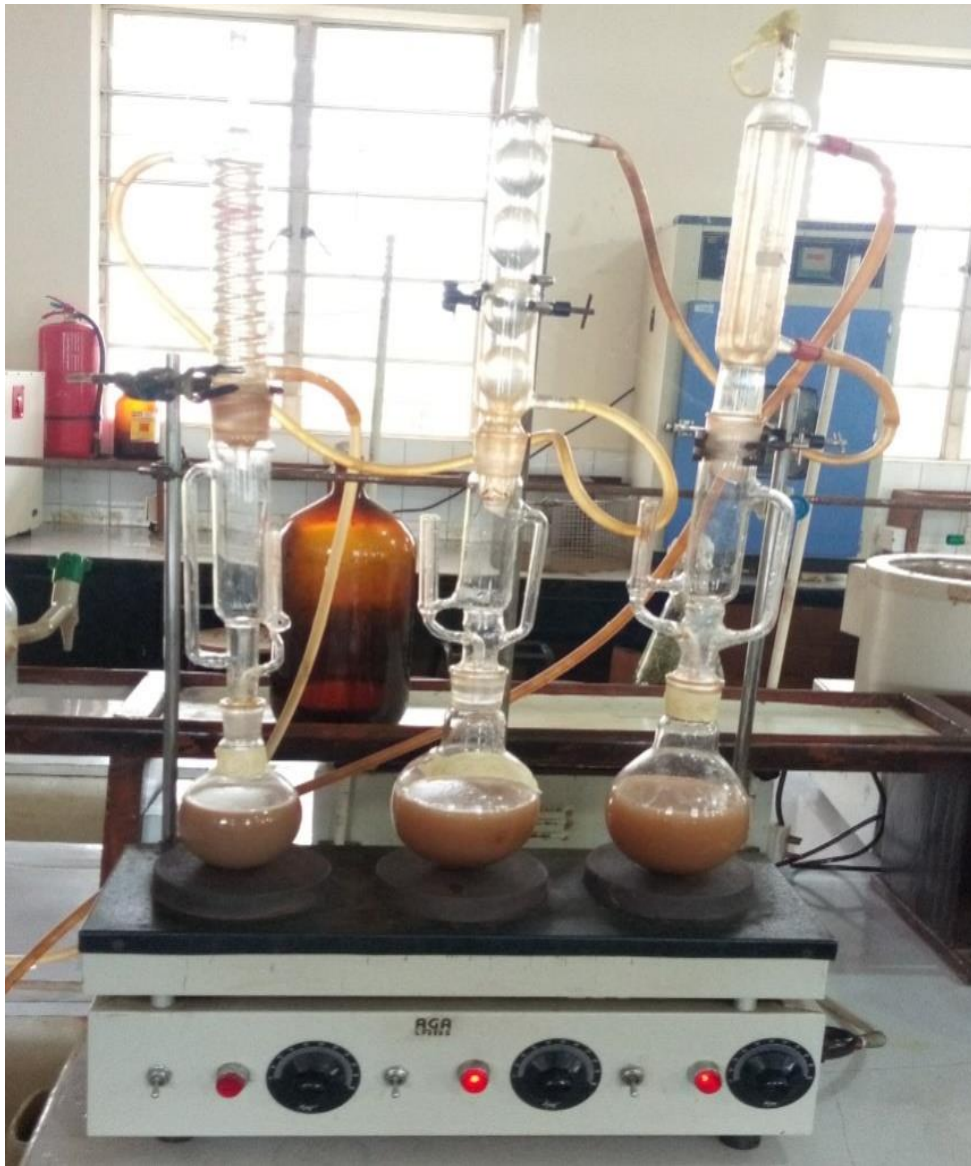
Appendix A13: Distillation apparatus used in extraction bioethanol
