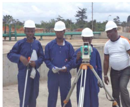
Plate IV: Demonstrating and surveying the use Reflectors and Digital Total station on site.
