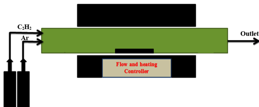
Figure 1. Schematic presentation of a CVD setup.
