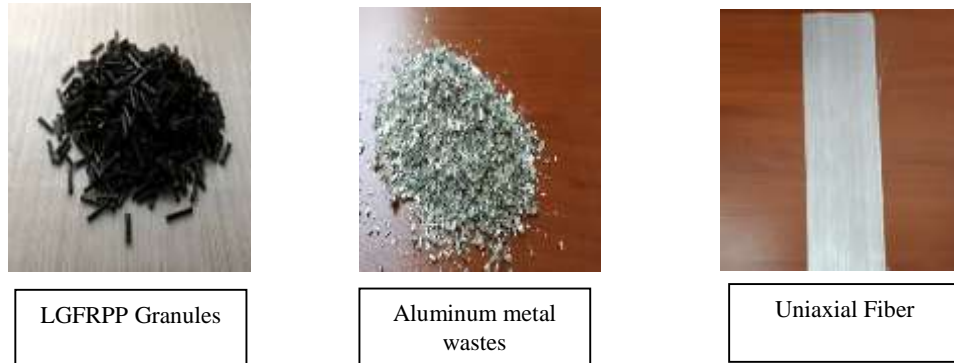
Figure 1. The materials used in manufacturing of composite
