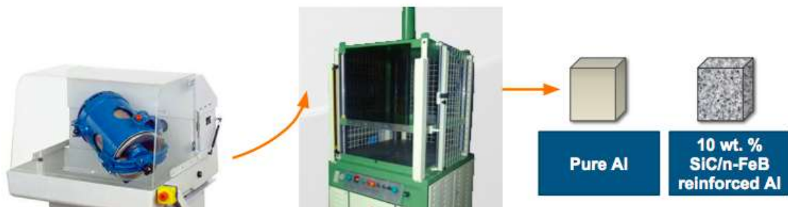
Figure 1. Schematic illustration of sample preparation
