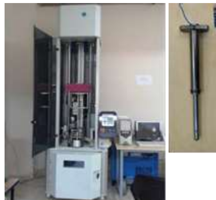
Figure 4. Low velocity impact testing machine and impactor
