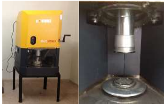
Figure 2. Gyratory press and compression head.
