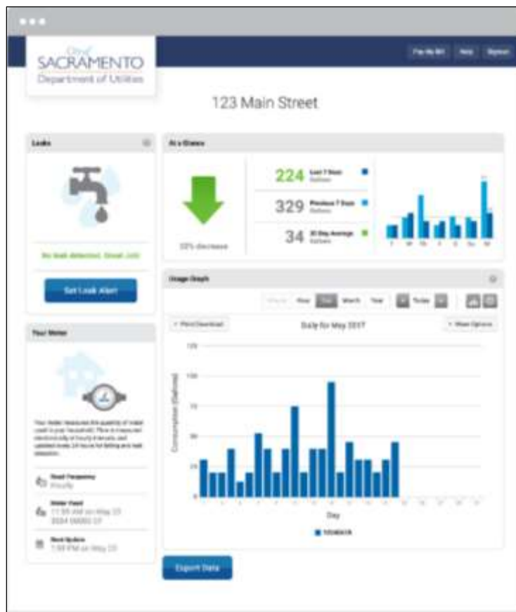
Figure 3. A screenshot of the developed customer application connected with smart meters [5]
