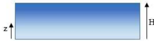
Figure 1. Illustration of FGM structure
