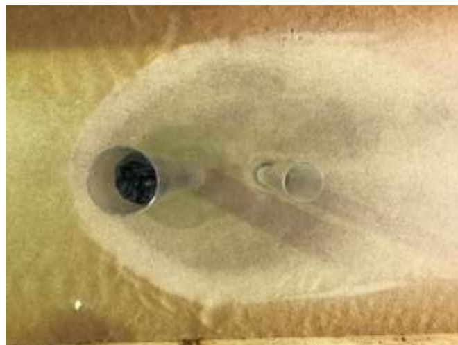
Figure 7. Scour after 144 hours
