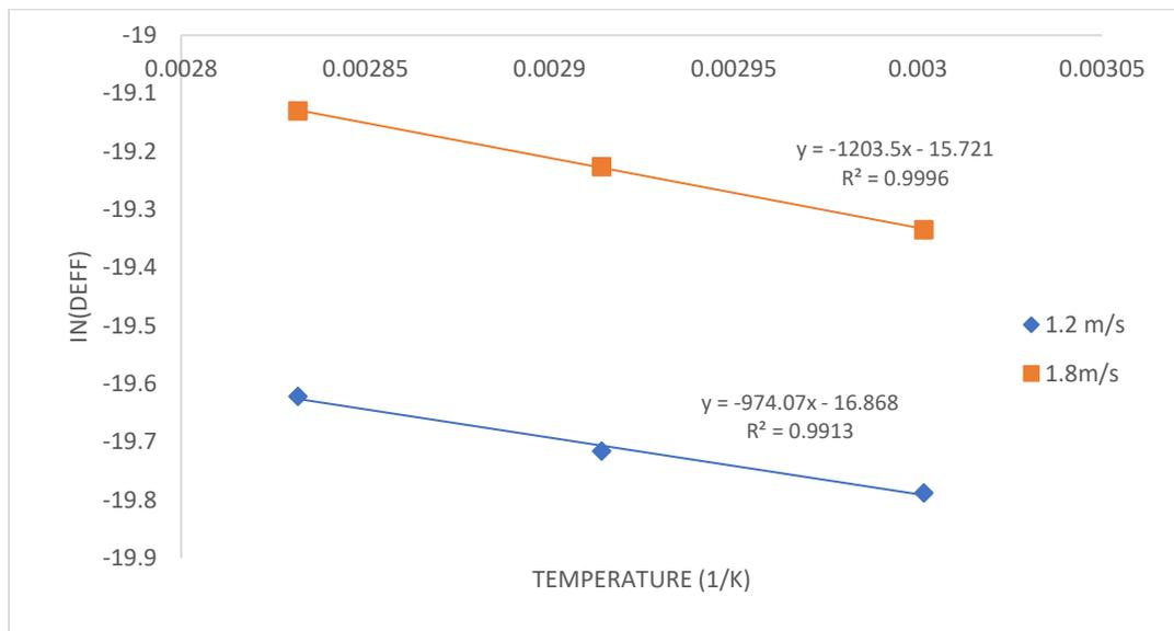
Figure 1: Relationship between effective coefficient moisture diffusivity and temperature for 1.2 and 1.8 m/s<sup>2</sup> air velocity.
