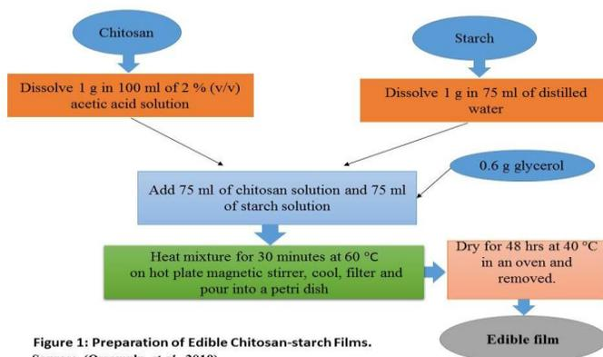
Figure 1: Preparation of Edible Chitosan-starch Films.
