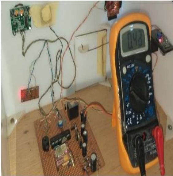
Figure 12: System Current Load Test
