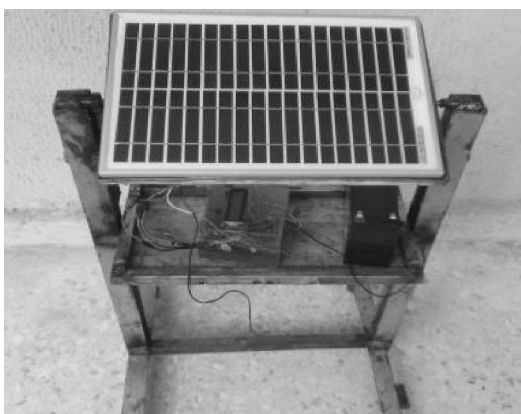
Figure 3.4: Solar tracking system
