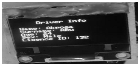
Figure 4. OLED Display of a Registered Driver's Information
