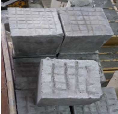
Figure 2 Roughness surface pattern of old PC specimens
