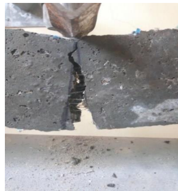
(b) Failure after Impact
