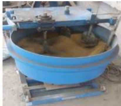
Figure 4: Revolving pan mixer for mixing fibrous concrete
