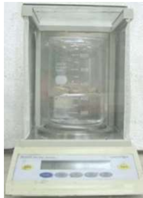
(b) Apparatus for density test (Mettler-Toldeo Balance)
