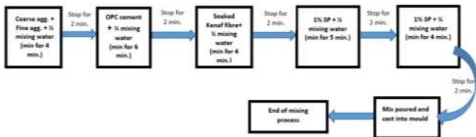
Figure 5: Mixing procedure for KBFCC
