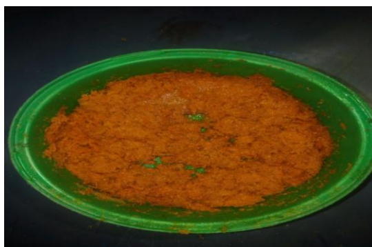
Plate 3: bamboo activated carbon impregnated with nitric acid ( \text{HNO}_3 ) Plate 4: bamboo activated carbon impregnated with \text{H}_2\text{SO}_4
