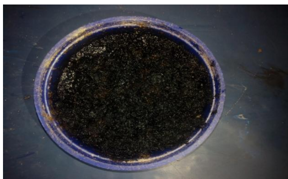
Plate 3: bamboo activated carbon impregnated with nitric acid ( \text{HNO}_3 ) Plate 4: bamboo activated carbon impregnated with \text{H}_2\text{SO}_4
