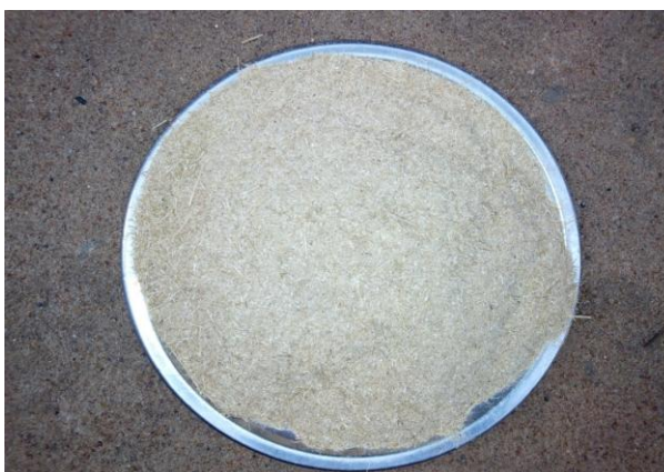
Plate 2: Crushed bamboo before impregnation
